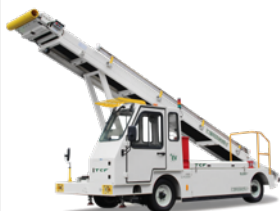
BLB80 散装货物装载机 Self-Propelled Conveyor Belt Loader
