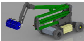
电动曲臂式飞机清洗车 Electric articulated aircraft cleaning platform
